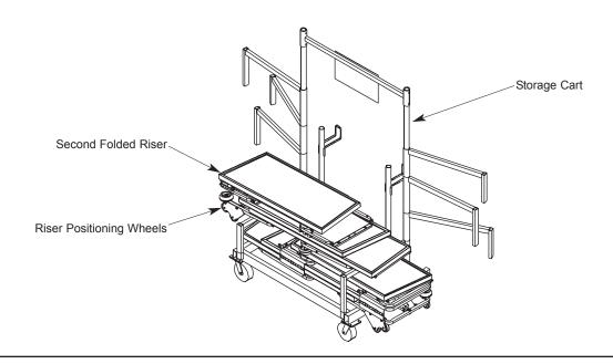
6. Close the two Swing Arms above the Riser. It will be necessary to lift all of the Arms high enough for the two Arms to clear the Riser.
